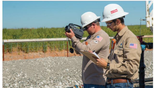
Employees operate a FLIR camera in Kingfisher, Oklahoma as they work to detect methane leaks.
