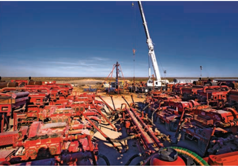
A wellsite becomes a hub of activity during fracture stimulation. Advanced completion techniques such as hydraulic fracturing have opened up new development opportunities in shale plays.
